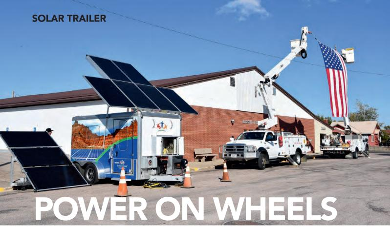
West Central Electric Cooperative's solar trailer serves as an interactive exhibit showcasing solar power generation in action for members. Equipped with a built-in generator, battery storage unit, inverter, and six rooftop solar arrays, the trailer is a great resource for public outreach and education efforts in South Dakota.
