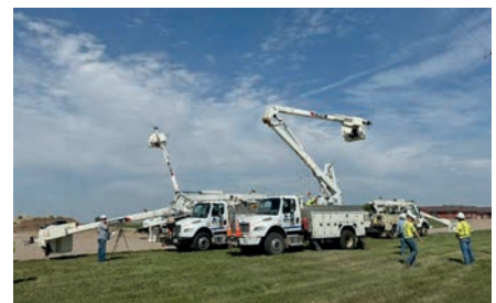
Crews perform annual dielectric testing on their trucks to ensure safety.
