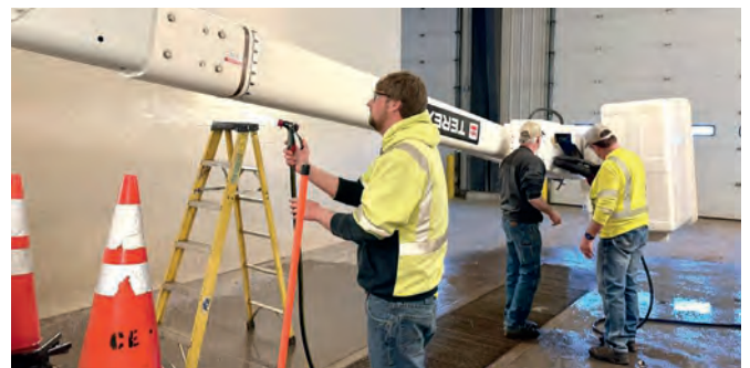
[REDACTED] washes the boom while [REDACTED] and [REDACTED] inspect hydraulic hoses and components.
